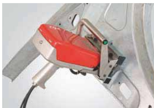
Custom clamping system / magnetic clamping
